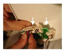
Replace the control panel and, place the handle.
