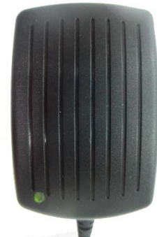
Battery Charger Fully Charged
