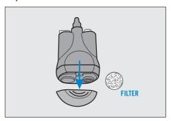
**Step 2.** Clean the filter and filter cover using clean fresh water only.
