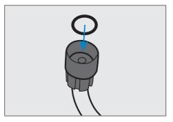
**Step 3.** Attach outlet connector to shower head and tighten by turning clockwise. Ensure a tight connection to avoid leakage.
