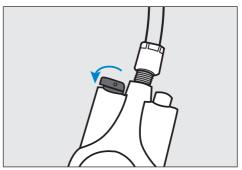
Insert USB charging cable into charging socket.
