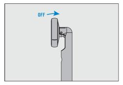
**Step 2.** Remove pump safety cap and push on/off switch to start the pump.
