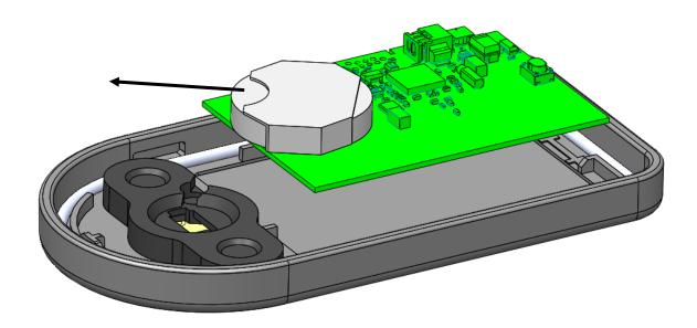
3. Place electronics board back into base. Pay attention to wire routing so that wires do not get pinched when lid is reassembled. Also check that the enclosure seal is properly seated into the base.
