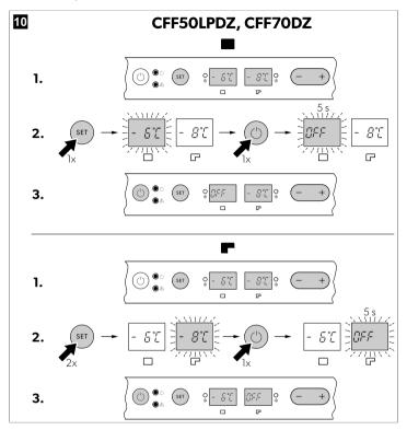
> Switch on the compartments (dual zone coolers).
