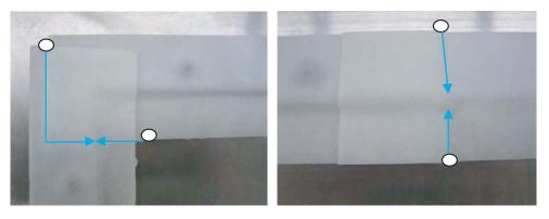
In the above images, the white circles indicate where 3M 4000UV should be applied in the corner and step situations. These two general categories can describe most common configurations. For configurations other than these, the general principle is to use  $3M^{TM}$  4000UV in any place where water (shown as blue arrows) could seep past an improperly joined overlap.
