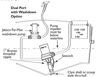
**Note:** For Model 209B a tee will need to be added to create an additional port for a washdown pump.
